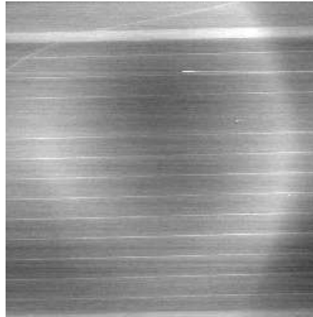
Figure 2.9: Panchromatic image of the waveguides in \text{Al}_2\text{O}_3:\text{Er} , with clearly visible charging effects.
