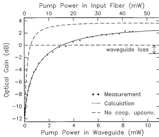
FIG. 2. Measurements of the (small-signal) optical gain at  $1.53 \mu\text{m}$  in a 4 cm long Er-doped ( $2.7 \times 10^{20} \text{ Er/cm}^2$ ) waveguide amplifier as a function of  $1.48 \mu\text{m}$  pump power. Calculations are included for two cases; with and without cooperative upconversion.
