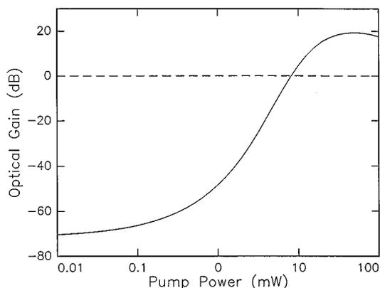
FIG. 4. Calculations of the optical gain at 1.53  $\mu\text{m}$  as a function of 1.48  $\mu\text{m}$  pump power in a 15 cm long waveguide amplifier doped with  $2.7 \times 10^{20}$   $\text{Er}/\text{cm}^3$  throughout the core of the waveguide.
