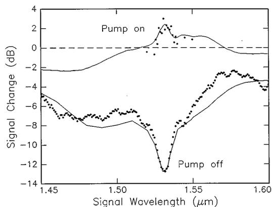
FIG. 3. Optical gain (9 mW 1.48  $\mu\text{m}$  pump on) and loss (pump off) spectra of a 4 cm long Er-doped waveguide amplifier (dots). Calculations of the spectra based on previously measured parameters (see Table I) are included as the solid lines.
