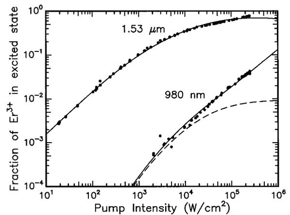
FIG. 5. Population fractions of  $\text{Er}^{3+}$  in the  ${}^4I_{13/2}$  state ( $1.53 \mu\text{m}$ ) and  ${}^4I_{11/2}$  state (980 nm) vs pump intensity for the low-concentration sample (0.12 at. % Er) on logarithmic scales (solid dots). The solid lines are fits to the data including effects of cooperative upconversion and excited state absorption. The dashed line shows the effect on the 980 nm luminescence of cooperative upconversion only.
