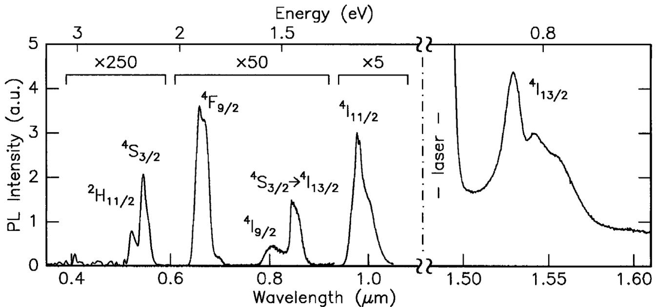
FIG. 2. Photoluminescence spectrum of an Er-implanted  $\text{Al}_2\text{O}_3$  ridge waveguide pumped with a  $1.48 \mu\text{m}$  laser diode. The transitions are indicated by their initial states. All but one of the transitions terminate at the ground state; the one exception is also indicated by its final state. Note the multiplication factors ( $\times 5$ ,  $\times 50$ ,  $\times 250$ ). The relative intensities may be compared.
