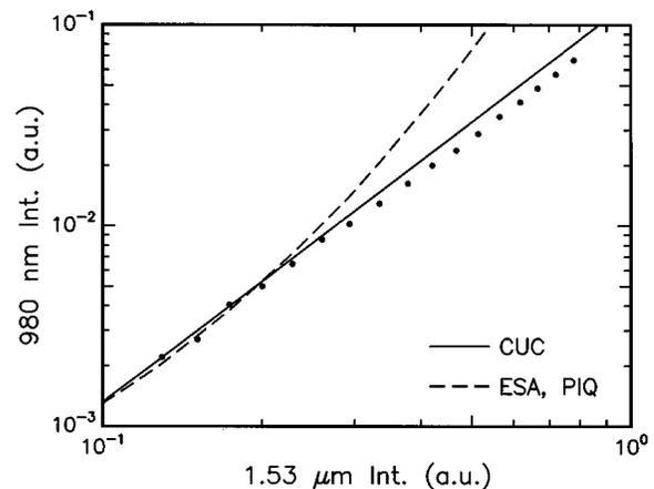
FIG. 3. Luminescence intensity at 980 nm vs that at  $1.53 \mu\text{m}$  for the high-concentration sample (1.4 at. % Er), on logarithmic scales (solid dots). The calculated behavior of three possible upconversion mechanisms is shown: cooperative upconversion (CUC), excited state absorption (ESA), and pair-induced quenching (PIQ).
