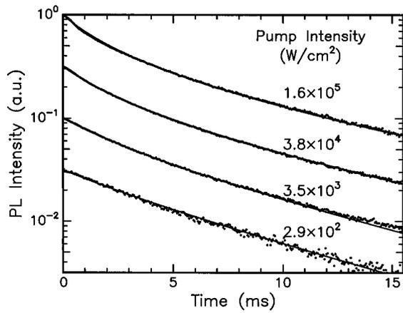
FIG. 6. Luminescence decay curves measured at  $1.53 \mu\text{m}$  (dots) after pumping to steady state and switching off the pump source for four different  $1.48 \mu\text{m}$  pump intensities. The curves are offset with respect to each other for clarity. The data are for the low-concentration sample (0.12 at. % Er). Fits to the data are shown as solid lines.
