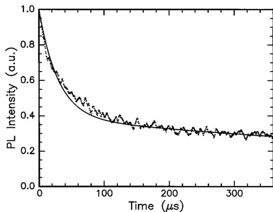
FIG. 7. Luminescence decay of the 980 nm luminescence (dots) after switching off the pump source for a pump intensity of  $5 \times 10^4 \text{ W}/\text{cm}^2$ . The data are for the low-concentration sample (0.12 at. % Er). The solid line is a fit to the data.
