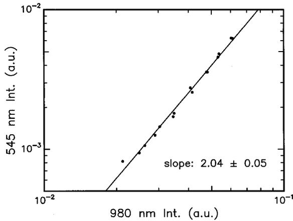
FIG. 4. Luminescence intensity at 545 nm vs that at 980 nm for the high-concentration sample (1.4 at. % Er), on logarithmic scales (solid dots). A linear fit through the data is shown.
