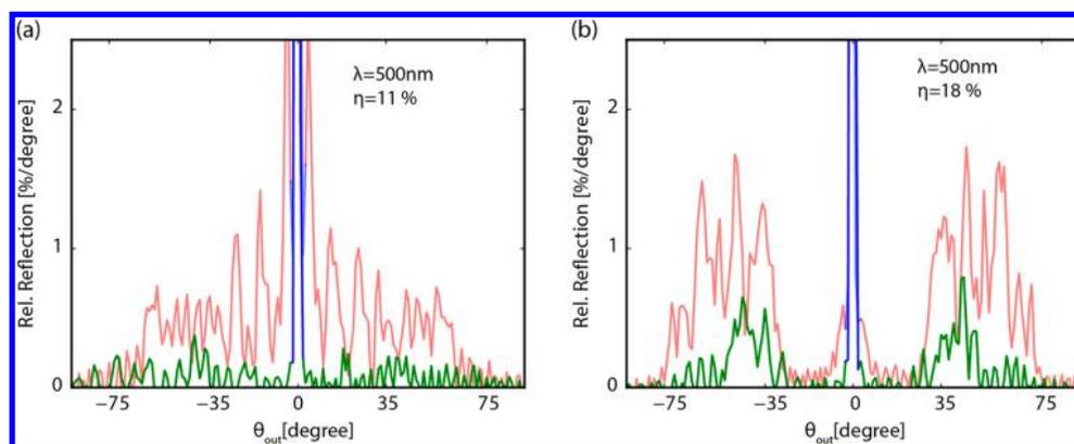
**Figure 6.** Measured angular reflection of the broad-angle reflector (a) and the large-angle reflector (b), off-resonance at  $\lambda = 500$  nm. Diffracted scattering (green) and specular reflection (blue) contributions are shown. Data for resonant excitation [ $\lambda = 650$  nm, same as Figures 4(d) and 5(d)] are overlaid for reference (red).
