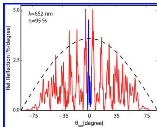
**Figure 3.** Broad-angle metasurface. Simulated angular scattering at  $\lambda = 652$  nm in the far field for the broad-angle metasurface illuminated at normal incidence composed of diffracted (red) and specularly reflected (blue) light. The dashed black line shows the angular profile of a perfect Lambertian diffuser.
